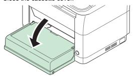
**Note** When storing the cassette, or when using paper larger than A4/Letter, remove the cassette cover.
